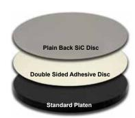
Double sided adhesive discs are adhered to a standard platen and used to secure plain back silicon carbide abrasive discs. Each provides 25-75 disc pulls depending on grit size, cycle time and force.
