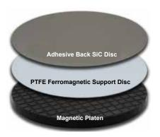
PTFE ferromagnetic support discs combine a PTFE surface with a rigid stainless steel disc. This allows adhesive backed abrasive discs/polishing cloths to be easily removed after use without any adhesive transfer. The nonslip backing keeps the disc in place even for coarse grinding.
